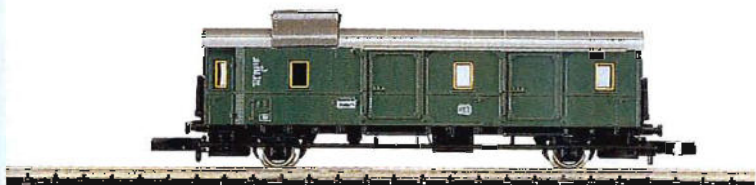
III 8752 "Thunder Box" Standard Design Baggage Car. Prototype: German Federal Railroad (DB) type D2ie. Model: Length over buffers 63 mm / 2-1/2".
