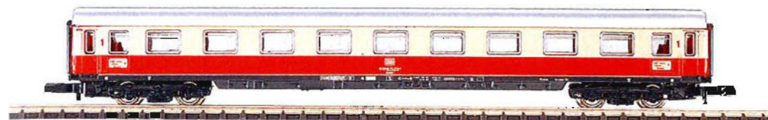
IV 8724 Express Train Passenger Car. Prototype: German Federal Railroad (DB) type Awmz 111. 1st class. Model: Length over buffers 120 mm / 4-3/4".
