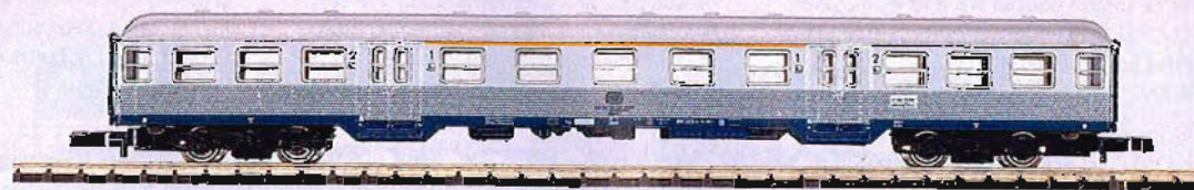
IV 8717 Commuter Car. Type Abnrzh 704. 1st and 2nd class. Length over buffers 120 mm (4-3/4").
