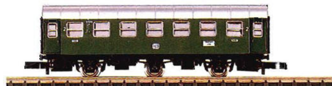
III 8707 Passenger Car. Type B3yge. 2nd class. Length over buffers 61 mm (2-3/8").
