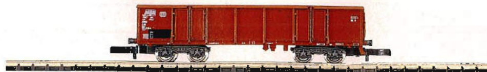
IV 8650 Gondola. Type Eaas 106. Length over buffers 63 mm (2-1/2").
