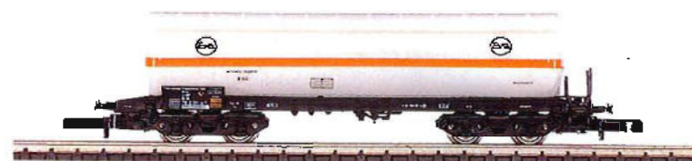
8608 Gas Tank Car with Heat Shield. Privately owned by EVA Company. Length over buffers 75 mm (3").
