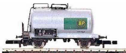
8614 Oil Tank Car. Privately owned by German BP, Inc. Length over buffers 40 mm (1-9/16").
