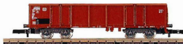
8650 Gondola. Eaos 106. Length over buffers 63 mm (2-1/2").
